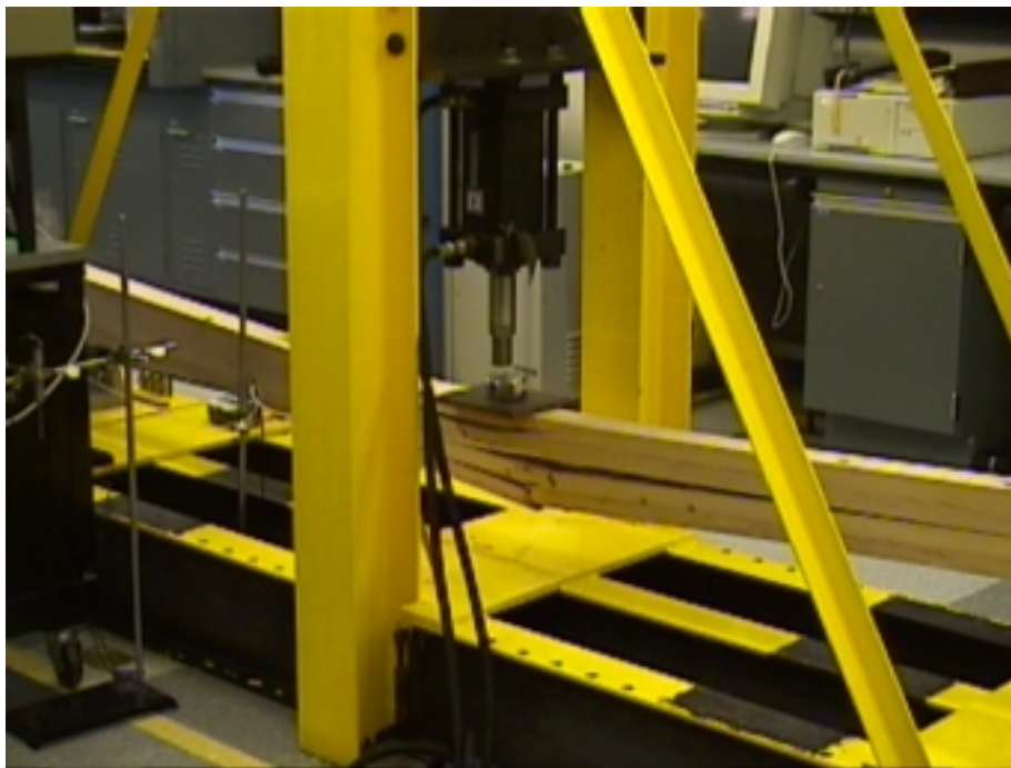
Figure 7. Static failure testing of 10-foot glulam section.
