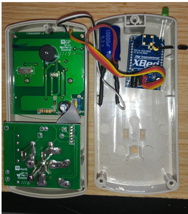
Figure 5c: Xbee interface to a Kill-A-Watt module
