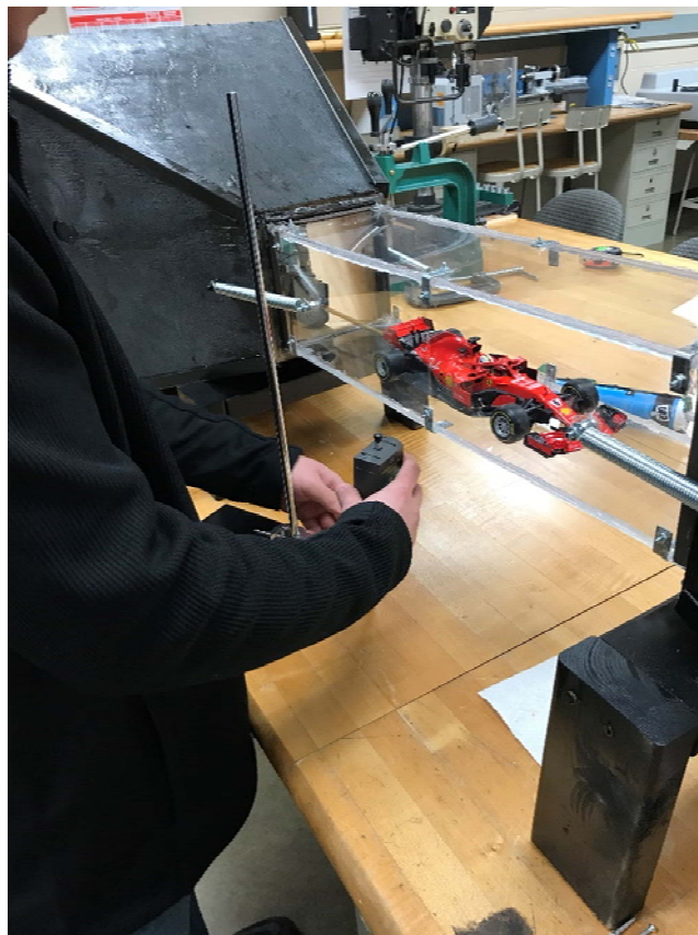
Figure 6. Model car tested inside the testing chamber with force sensors being installed underneath the car and behind it to measure the down and drag forces respectively
