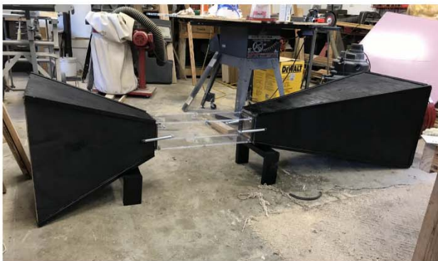
Figure 2. Finalized built-up wind tunnel
