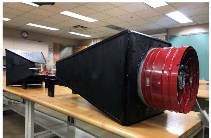
Figure 2. Finalized built-up wind tunnel
