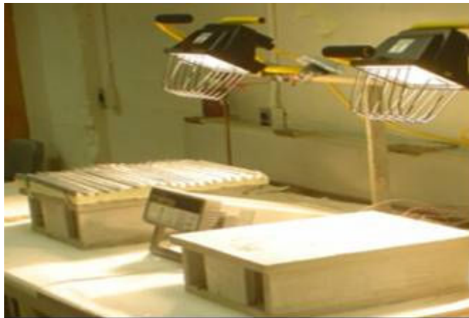
Figure 2. Two insulation systems on top of identical structures under two 500-watt lamps
