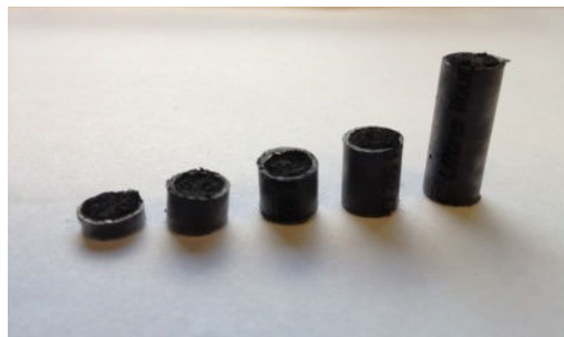
Figure 1: Dry ECNF samples – cylinders packed with ECNF, 0.25 cm to 2 cm
