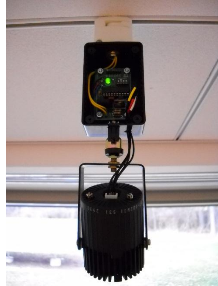
Figure 6. LED Spotlight System Breadboard and Final Assembly
