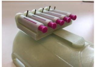
Figure 3: 3D printed IFC mechanism attached to gauntlet
