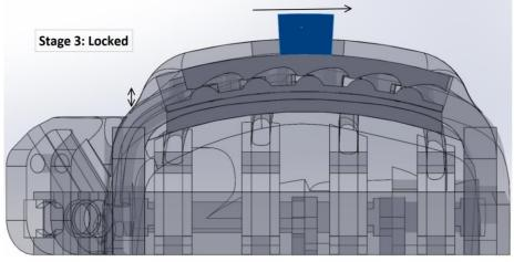
Figure 7: Grip locking mechanism locked
