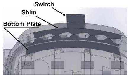
Figure 4: Grip lock mechanism
