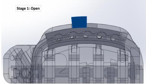
Figure 5: Grip Locking Mechanism open (unlocked)
