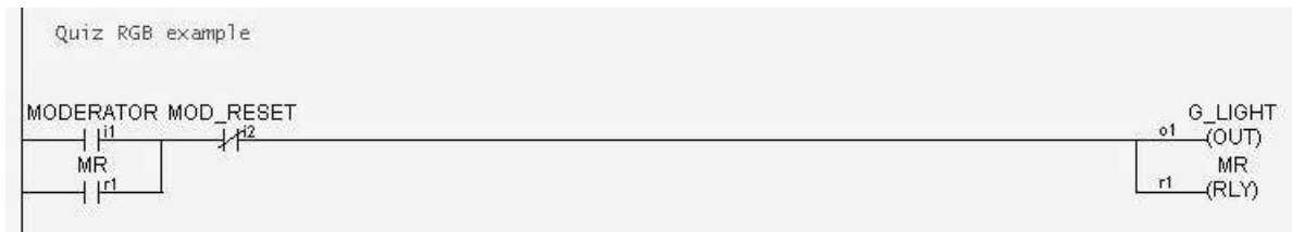
Figure 6. First rung of the i-TRiLOGI program latching the green light once the moderator button is pressed.
