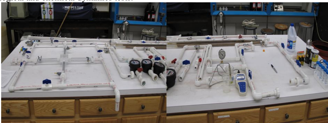
Figure 1. PVC Based Pipe System Components as Assembly Blocks for Lab Exercises
