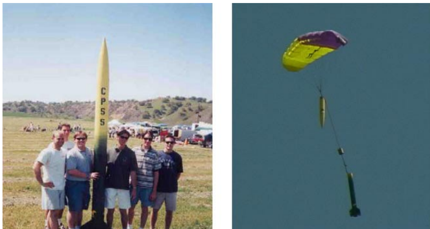
Figure 1 – High Power Rocket with Parafoil Recovery System
