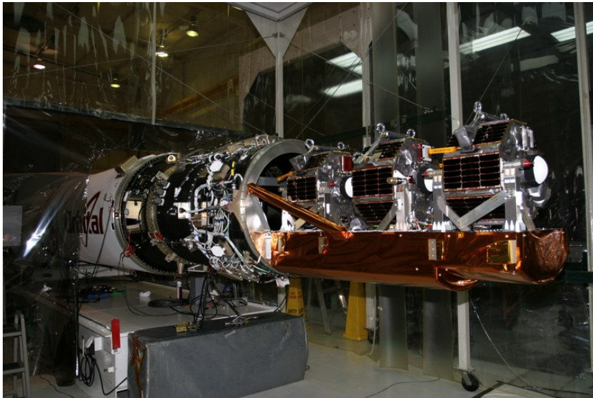
Figure 1: Three ST-5 Spacecraft on Pegasus XL launch vehicle, being lifted on March 11, 2006.
