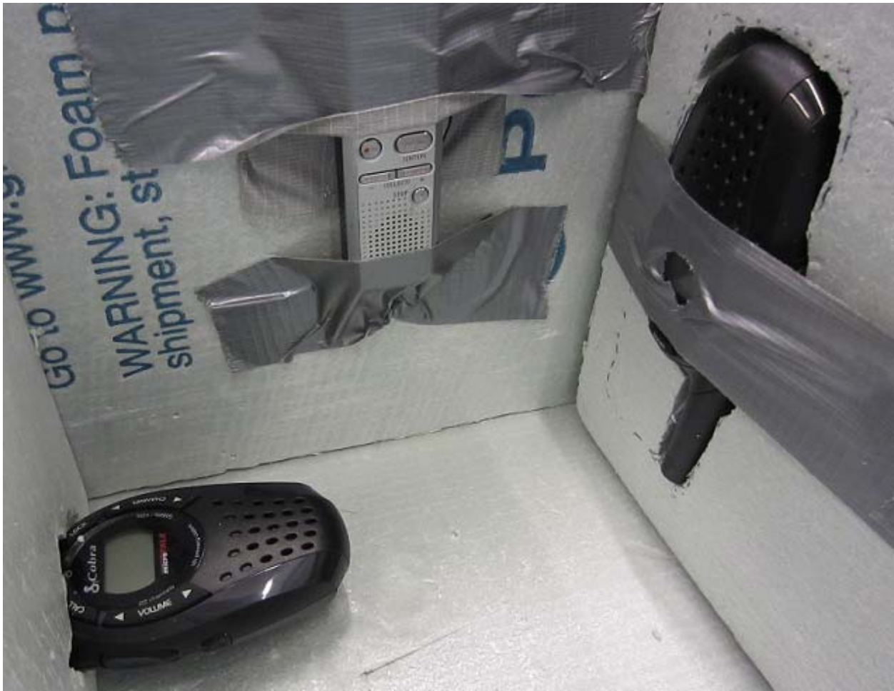
Figure 2. Orientation and position of radios 2 and 3, plus voice recorder, inside payload vessel.
