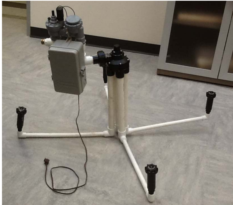
Figure 7. Portable sprinkler system
