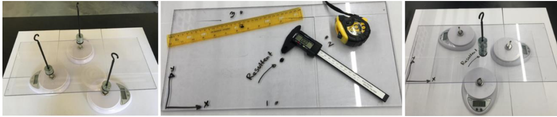
Figure 9: Demonstration of a vector cross product with an equivalent force-couple system using the experimental kit.
