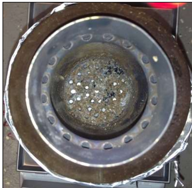
Figure 5: The gasifier's inner container, where fuel is retained, was imaged after a burn sequence to show the trace amount of ash remaining.
