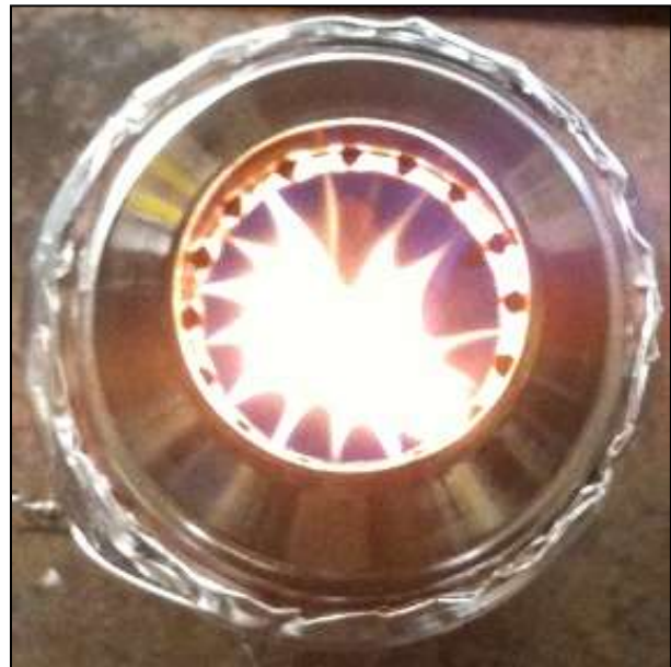
Figure 3: A top-down view of the gasifier reveals a star-shaped combustion pattern aligning with holes drilled in the thermos throat to enable mixing of air and syngas. This pattern proves the syngas (and not the wood chips in the thermos) is burning.
